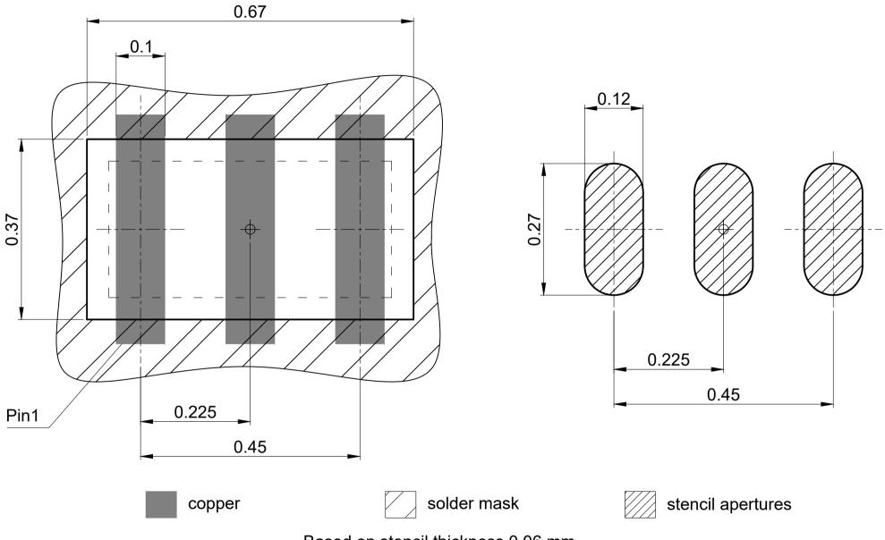
Based on stencil thickness 0.06 mm All undimensioned radii 0.06 All dimensions are in units mm
