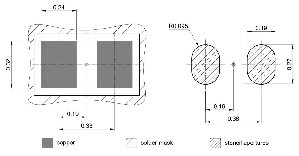
Based on stencil thickness 0.08 mm All dimensions are in units mm
