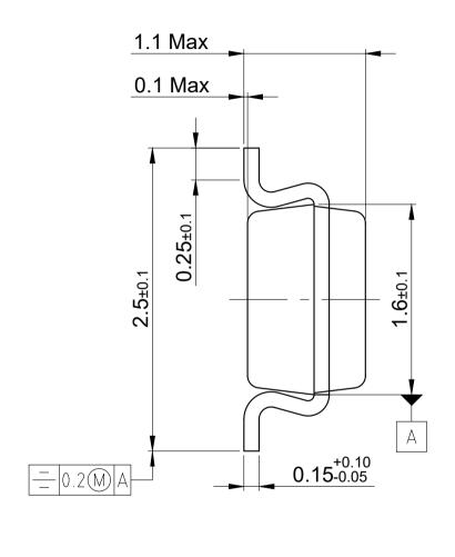
Note: Mold flash, protrusions or gate burrs of 0.2 mm maximum per side are not included 1) Contour of slot depends on profile of gull-wing lead form All dimensions are in units mm
