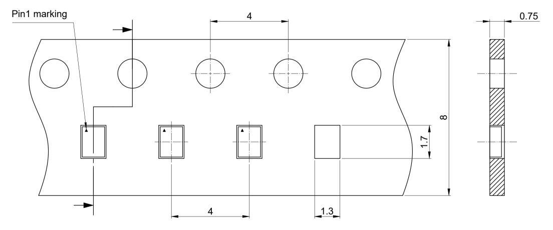
All dimensions are in units mm The drawing is in compliance with ISO 128-30, Projection Method 1 [ $\bigcirc \oplus$ ]
