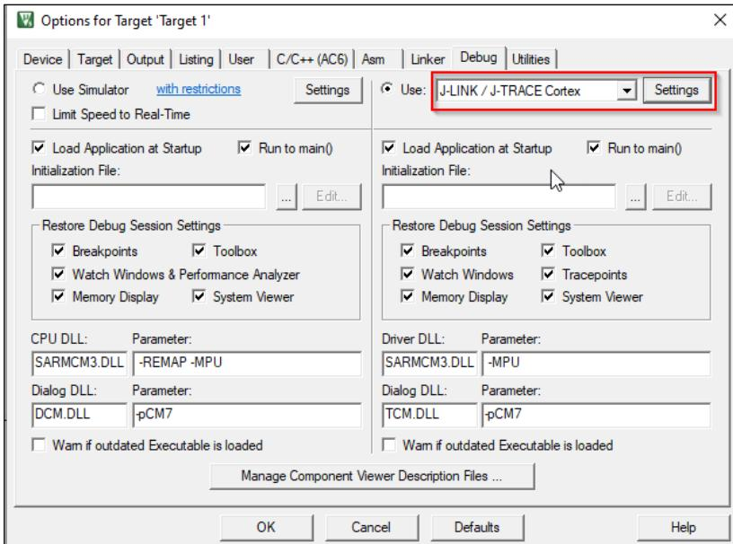
2. On the **Debug** tab in the **Target Driver Setup** dialog:
