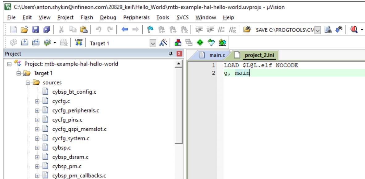
15. Select **Project > Build Target** to build the application and execute post-build commands.
