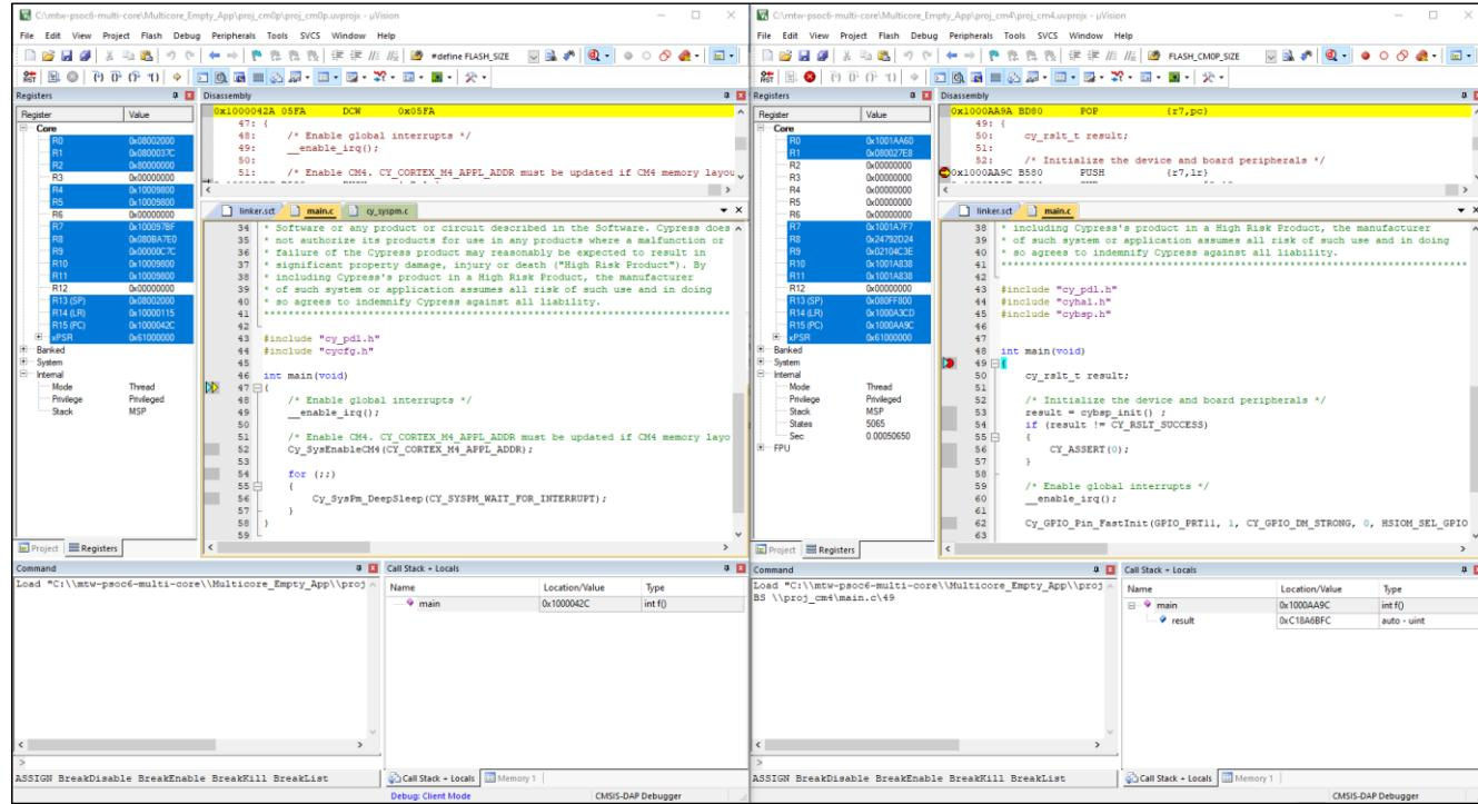
The left side of the screen shows a µVision IDE instance attached to the CM0+ core. The right side shows the CM4 core has not started yet. Once the `Cy_SysEnableCM4()` function on the CM0+ core has been executed, the CM4 will start executing its application. You can step through the code by switching back and forth between the two µVision IDE instances.
