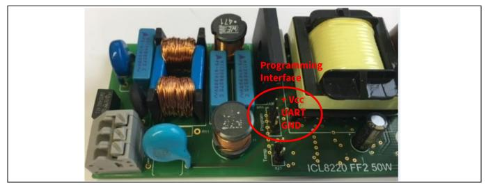
Figure 3 Connection between the .dp Interface Gen2 and the XDPL8220 reference board
