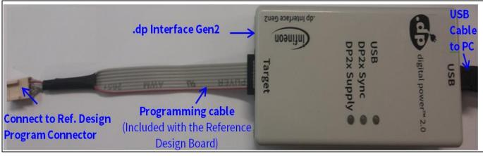
Figure 2 .dp Interface Gen2 connection
