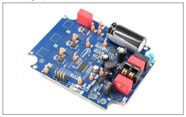
The EVAL\_DRIVE\_3PH\_PFD7 is a complete evaluation board for motor drive applications. The kit demonstrates Infineon's latest discrete power SJ MOSFET CoolMOS™ PFD7 technology for motor drive applications.
