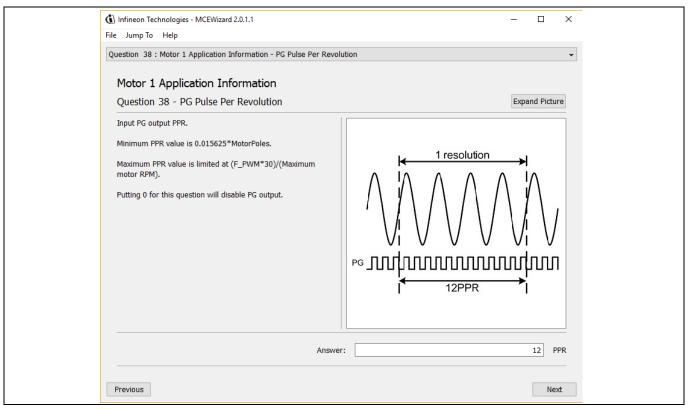
Figure 33 PG pulse per revolution configuration
