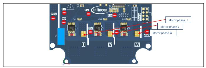
Figure 13 Motor-side connector
