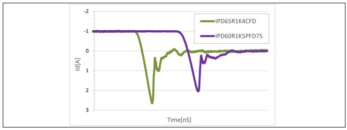
Figure 3 Reverse recovery charge Qrr comparison for different CoolMOS™ fast body diode technologies at 1A freewheeling current, dV/dt less than 5 V/ns ,T<sub>amb</sub> = 25°C
