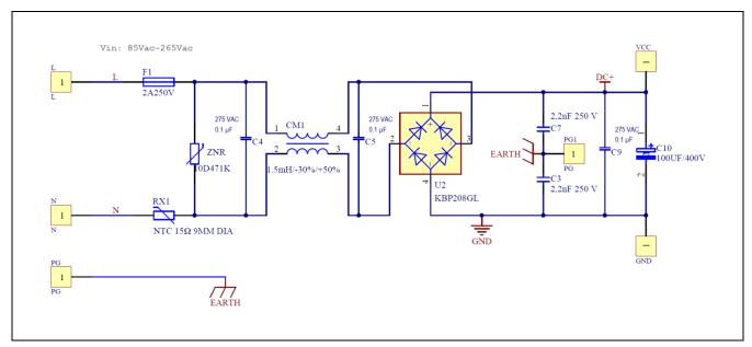
Figure 21 Schematic for EMI input filter and AC-DC section of the EVAL\_DRIVE\_3PH\_PFD7
