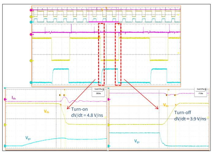
Figure 23 Controlled dV/dt
