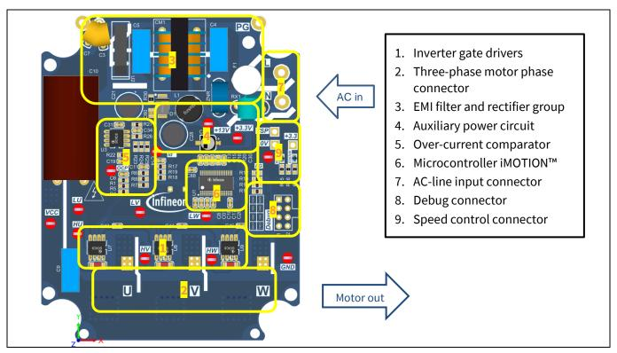
Figure 10 Functional groups of the EVAL\_DRIVE\_3PH\_PFD7 evaluation board's top side
