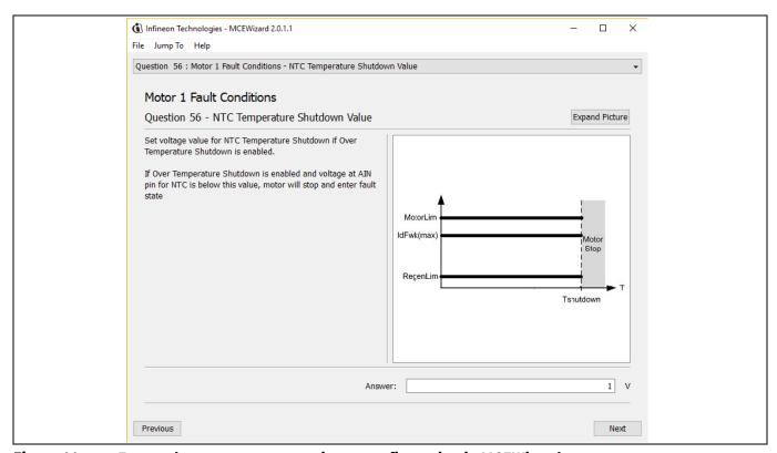
Figure 32 External temperature sense input configuration in MCEWizard
