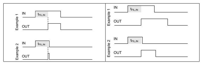
Figure 27 Typical input filter
