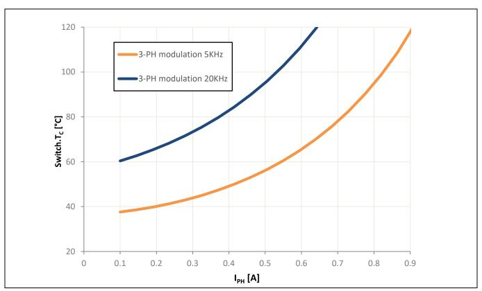
Figure 9 Thermal characterization, at 5 to 20 kHz
