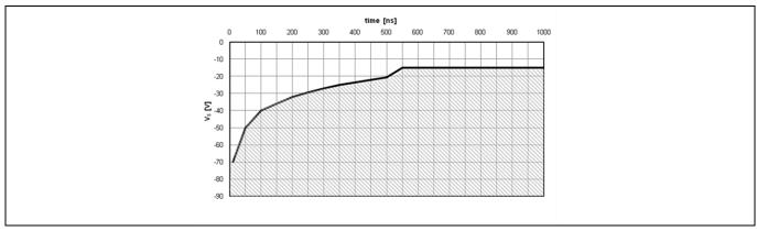
Figure 30 Negative VS transient SOA for 2ED28073J06F @ VBS=15 V
