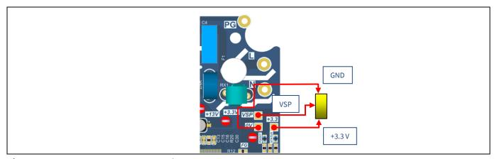
Figure 14 Speed control potentiometer connector
