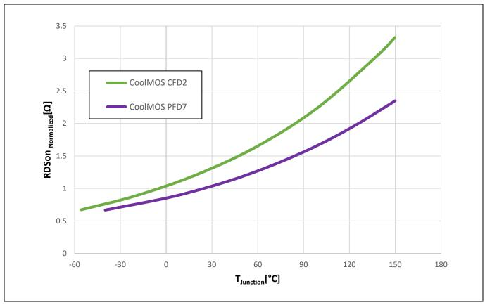
Figure 5 Temperature dependency of the R<sub>DS(on)</sub> CoolMOS<sup>™</sup> CFD2 vs. PFD7
