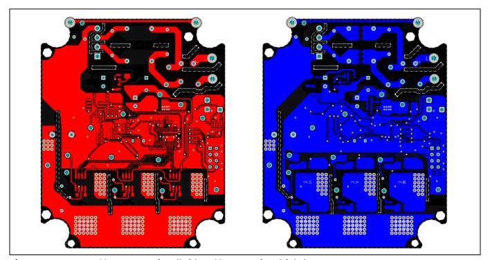
Board layout top view (left) and bottom view (right) Figure 37
