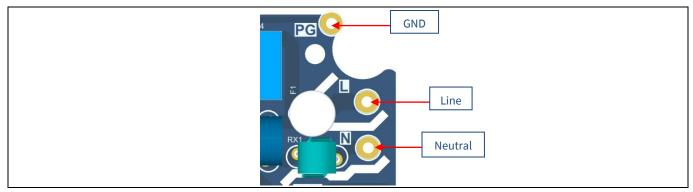
Figure 12 AC-line connector
