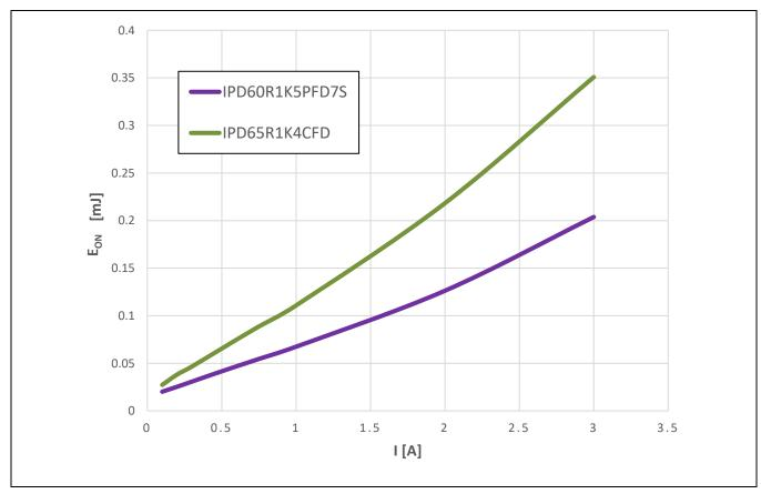
Figure 4 Turn-on loss comparison with different CoolMOS™ fast body diode technologies at 320 V DC, gate voltage 15 V, dV/dt less than 5 V/ns ,T<sub>amb</sub> = 25°C (at the same R<sub>g</sub>)
