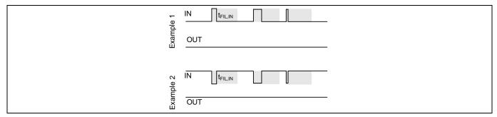
Figure 29 Noise rejecting input filters
