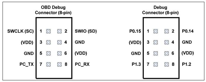
Figure 15 Pin assignment of the eight-pin debug connector
