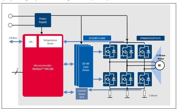
Figure 1 EVAL\_DRIVE\_3PH\_PFD7 block diagram
