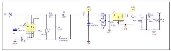
Figure 24 Power supply section of the EVAL\_DRIVE\_3PH\_PFD7 evaluation board
