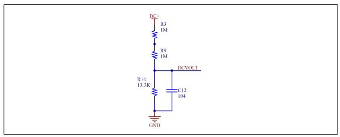
Figure 26 The DC bus sense resistor on the EVAL\_DRIVE\_3PH\_PFD7 evaluation board
