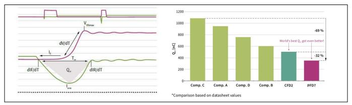
Figure 2 Highest reliability from lowest reverse-recovery charge and reverse-recovery time
