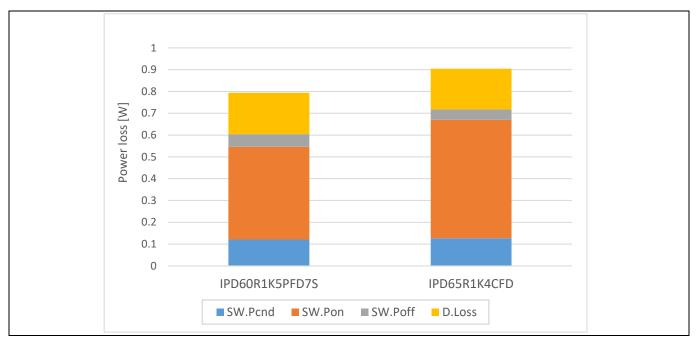
Figure 6 Estimated distribution of losses for different CoolMOS™ fast body diode technologies: 320 V input at 20 kHz, T<sub>i</sub> = 100°C, switching current = 0.5 A (same dV/dt less than 5 V/ns)
