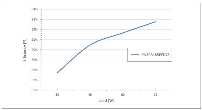
Figure 36 Efficiency measurement curve f<sub>\_sw</sub> = 10 kHz, IPN60R1K5PFD7S
