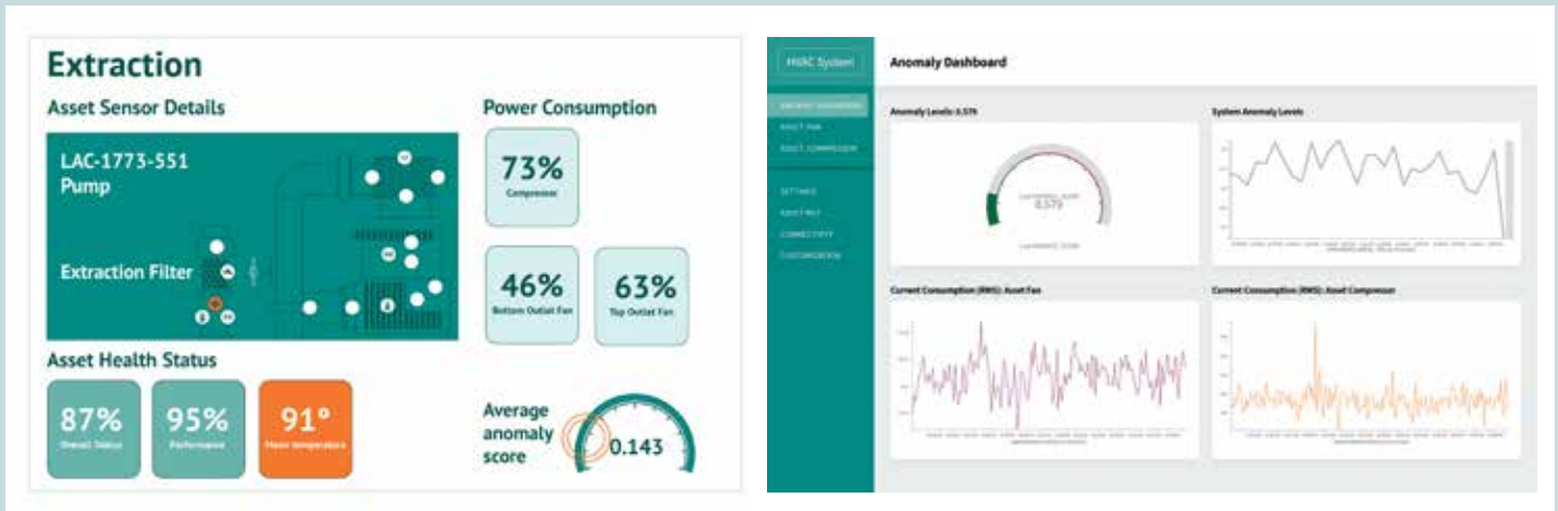
Figure 3: With PdM implemented, dashboards provide a quick overview of the status of devices and systems.
