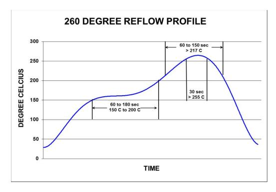
This part is compliant with EU Directive 2011/65/EU (RoHS Directive) and does not contain lead, mercury, cadmium (0.01%), hexavalent chromium, PBB or PBDE in concentrations greater than 0.1%, except as permitted by Annex III. Further part complies with 3 reflow cycles per JEDEC J-STD-020
