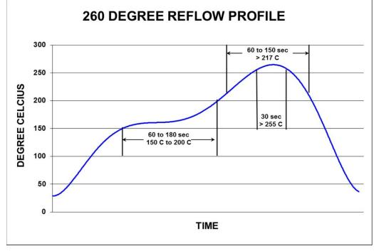
This part is compliant with EU Directive 2011/65/EU (RoHS Directive) and does not contain lead, mercury, cadmium (0.01%), hexavalent chromium, PBB or PBDE in concentrations greater than 0.1%, except as permitted by Annex III. Further part complies with 3 reflow cycles per JEDEC J-STD-020
