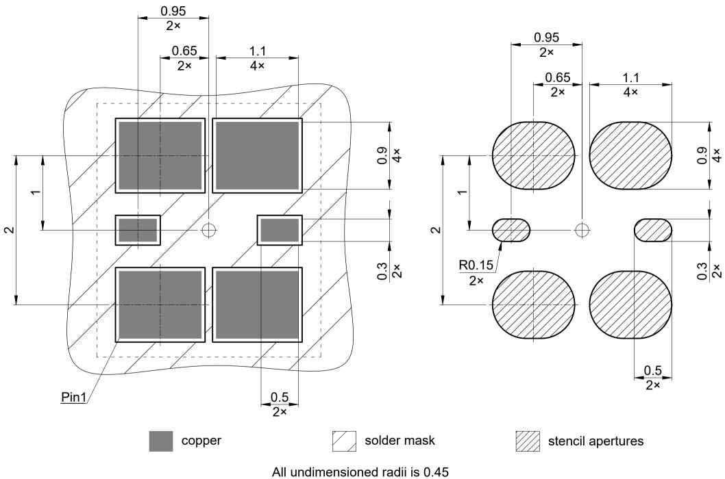
All dimensioned radii is 0.45 All dimensions are in units mm
