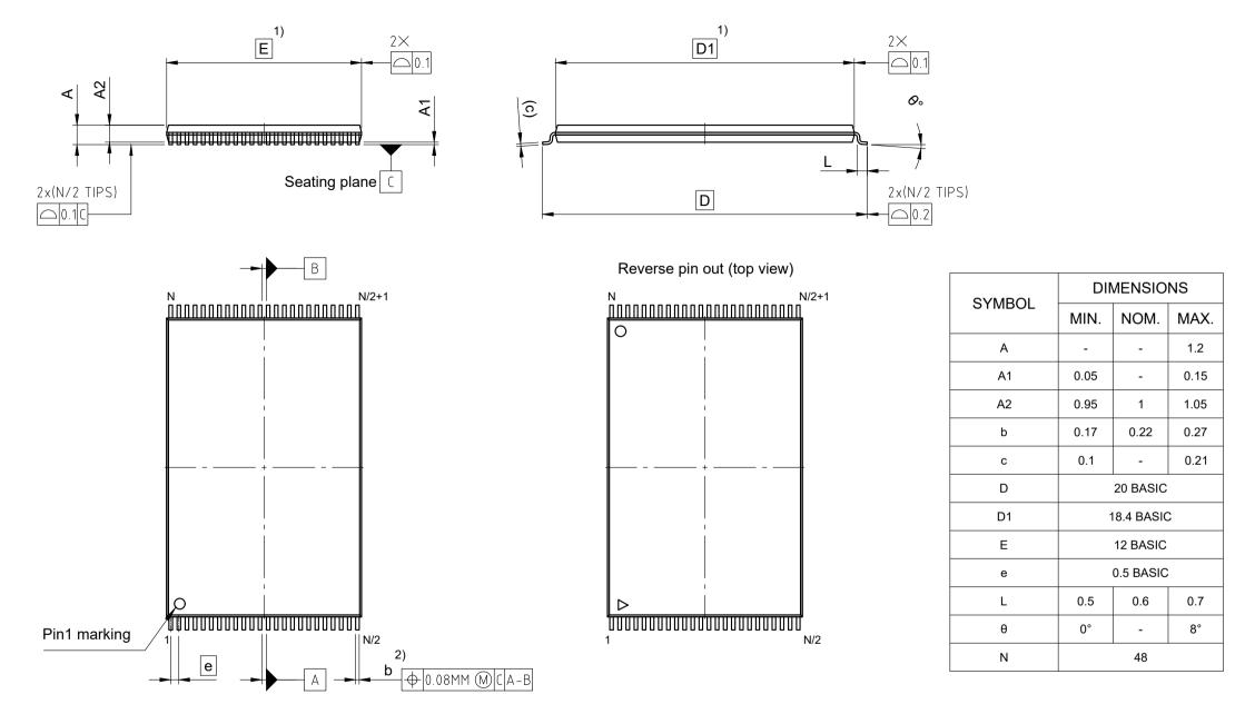
1)Dimensions D1 and E do not include mold protrusion. allowable mold protrusion on E is 0.15mm per side and on D1 is 0.25mm per side.
