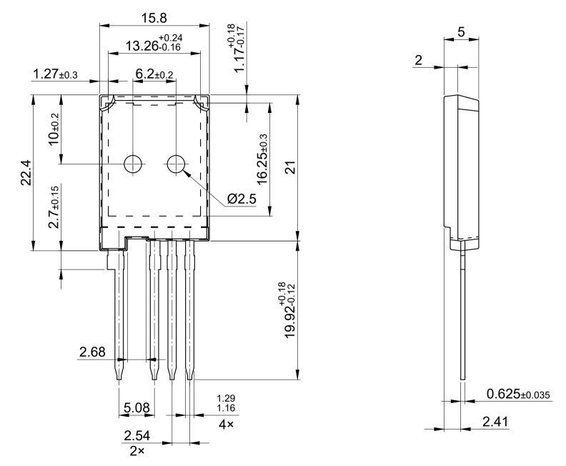
1) All dimensions refer to JEDEC standard TO-247 do not include mold flash or protrusions All dimensions are in units mm
