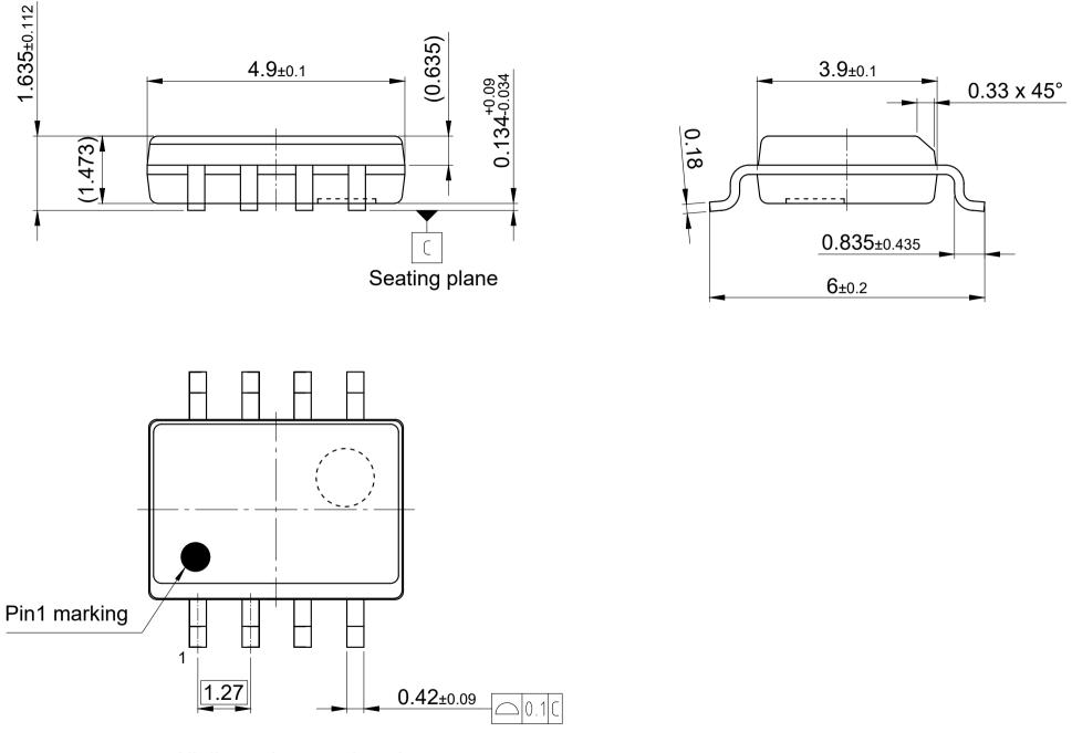
All dimensions are in units mm The drawing is in compliance with ISO 128-30, Projection Method 1 [ $\bigcirc \phi$ ] Drawing according to ISO 8015, general tolerances ISO 2768-mK
