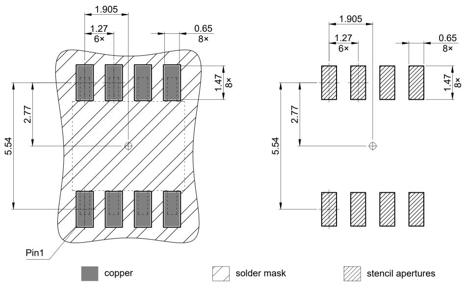
All pads are non-solder mask defined All dimensions are in units mm
