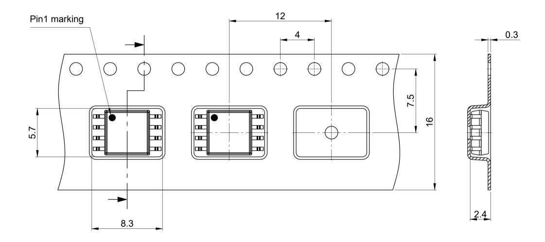
All dimensions are in units mm The drawing is in compliance with ISO 128-30, Projection Method 1 [ $\bigcirc \oplus$ ]
