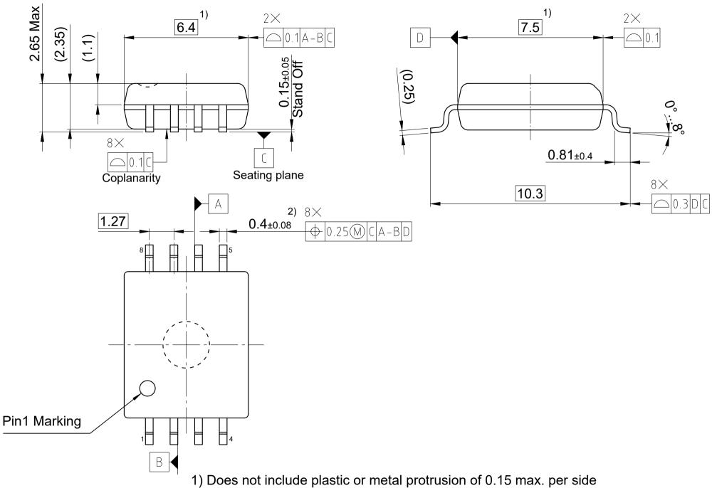
2) Dambar protrusion shall be maximum 0.1mm total in excess of lead width All dimensions are in units mm
