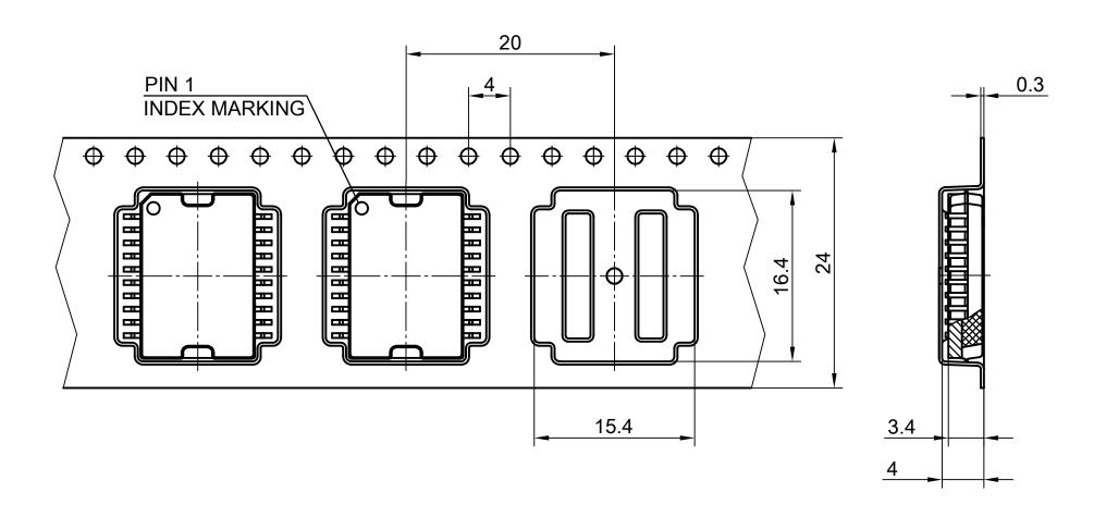
ALL DIMENSIONS ARE IN UNITS MM THE DRAWING IS IN COMPLIANCE WITH ISO 128 & PROJECTION METHOD 1 [  $\rightleftharpoons$  ]
