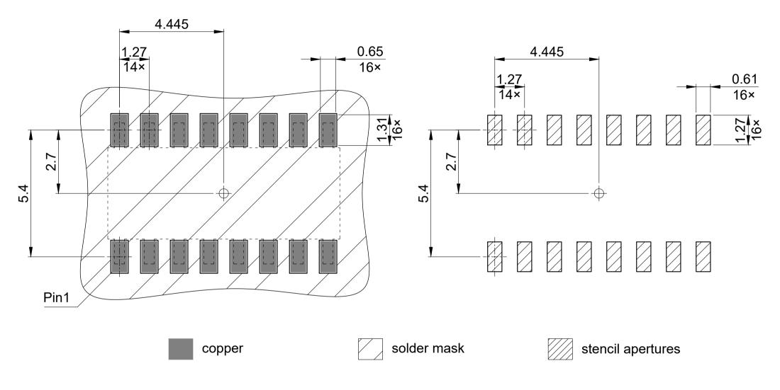
All pads are non-solder mask defined All dimensions are in units mm
