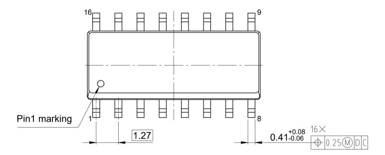
1) Does not include plastic or metal protrusion of 0.25 max. per side All dimensions are in units mm
