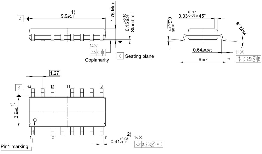
1) Does not include plastic or metal protrusion of 0.15 max. per side
